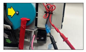
If it is not receiving at least **18v**, then there is a fault with the PCB or Toggle Switch, follow 'is the toggle switch receiving power' testing guide.
