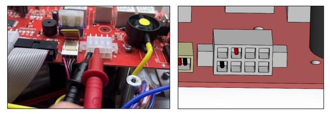
If the toggle switch port is not receiving at least **18v**, then there is a fault in the board. The board must be replaced.
