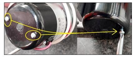
Inspect the lift motor brushes, they should be held in place by a spring as shown below. If the brushes have popped out (as shown), reposition the brushes in place and secure with the spring. There are two brushes inside the motor. Make sure both are refitted correctly.
