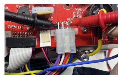
If the toggle switch port is not receiving at least **18v**, then there is a fault with the toggle switch. The toggle switch must be replaced.
