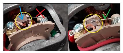
Once the brushes are positioned back in place. Secure the lift motor cap back in place with the pozi-pan screws.
