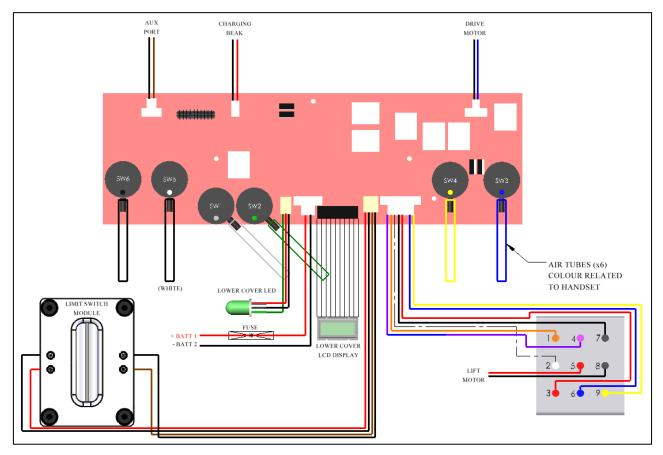
Each of the below troubleshooting guides requires a multi-meter to test power inputs and outputs from the board. Prepare the multi-meter by setting it to read DC volts, the red lead (positive) should be plugged into the voltage port, and the black lead (negative) should be plugged into the COM port. The display screen should show a reading of 0.0 volts.
