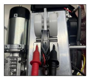
If the auxiliary beak is not receiving at least 17v, then there is a fault with the auxiliary beak. The beak must be replaced.
