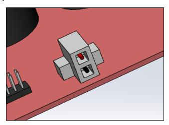
If the auxiliary port is not receiving at least 18v, then there is a fault in the board. The board must be replaced.
