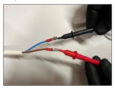
If the auxiliary coiled cable is not receiving at least 17**v**, then there is a fault with the coiled cable. The coiled cable must be replaced.
