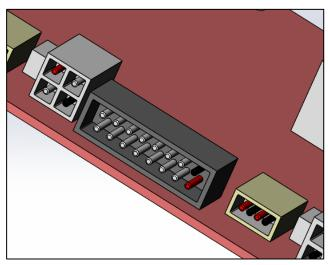
If the LCD port is not receiving at least 4.5v, then there is a fault in the board. The board must be replaced.
