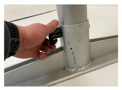
Step 3 – Raise the Leg from its fixing within the foot.
