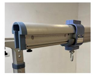
Step 5 – Traverse the Trolley from the track where the end stop has been removed.
