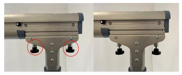
Step 3 – Loosen the two star handles at the opposite leg post to release the track from its fixing.
