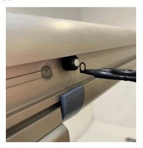
Step 2 – Remove the rubber bung from the pin.
