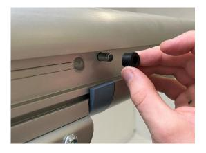
**3.** Remove the pin to release the trolley from the track.
