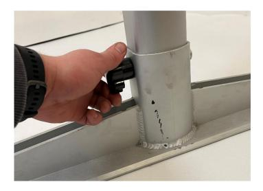
3. Raise the support post from its fixing within the foot.
