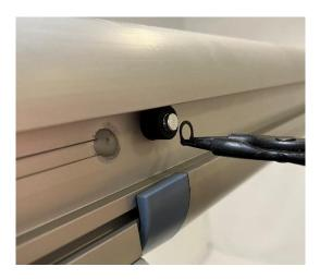
2. Remove the rubber bung from the pin.
