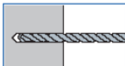
1. Drill hole to correct diameter and depth for stud size being used.
