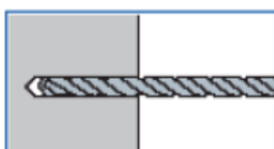
1. Drill hole to correct diameter and depth for stud size being used.
