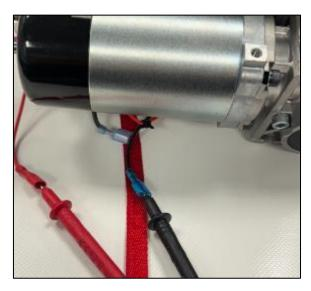
If it is not receiving at least **18v**, then there is a fault with the PCB or Toggle Switch, follow 'is the toggle switch receiving power' testing guide.
