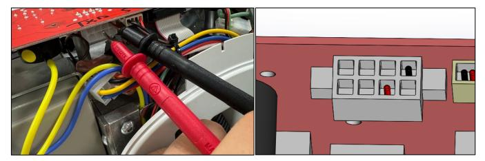
If the toggle switch port is not receiving at least **18v**, then there is a fault in the board. The board must be replaced.
