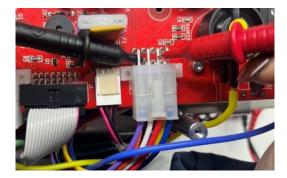
If the toggle switch port is not receiving at least **18v**, then there is a fault with the toggle switch. The toggle switch must be replaced.
