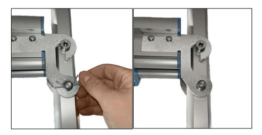
2. Remove the track pin from its fixing point.
