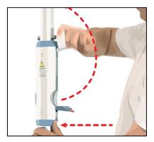
6. Push the top part of the support post upwards until the top plate compresses against the ceiling. Push until you hear two clicks on the ratchet
