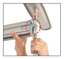
13. Extend or contract the track to fit between the two support posts and hook it on to the support post pins at the other side.
