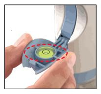
8. Pull the lever down until it flat to the support leg and click into place
